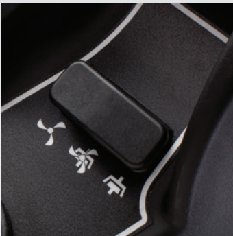
C Series tractors feature a push-button controlled power take-off for driving accessories
